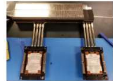
3. Previously installed indium foil removed & heat sinks reinstalled, bare chip to heat sink contact
