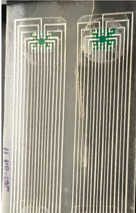
Specimen with more traces and tight pitch spacing
