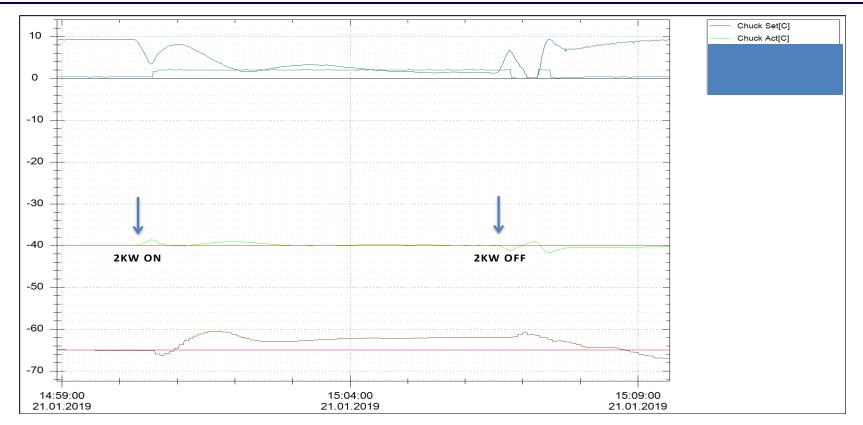
Able to dissipate 2KW – Temperature control within 2K
