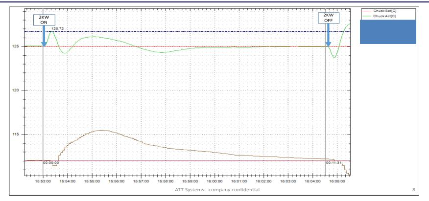
Able to dissipate 2KW – Temperature control within 2K
