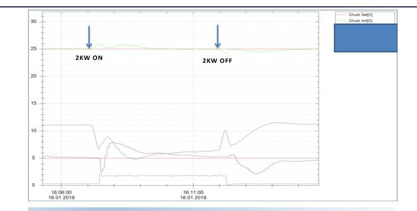
Able to dissipate 2KW – Temperature control within 1K
