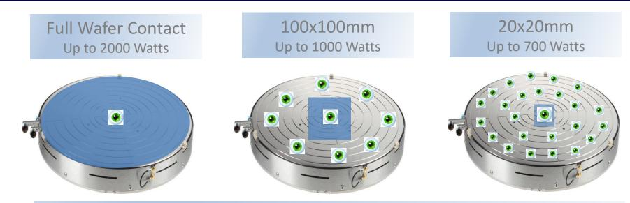
For Full Wafer Contact applications one control sensor is enough Smaller contact areas require multiple control sensors to detect temp changes Number of in-built sensors is limited due to chuck complexity Number of AddOn sensors is scalable, currently up to 25 sensors Requires advanced temp control algorithms
