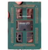
Split by function: I/O and Memory Controller
